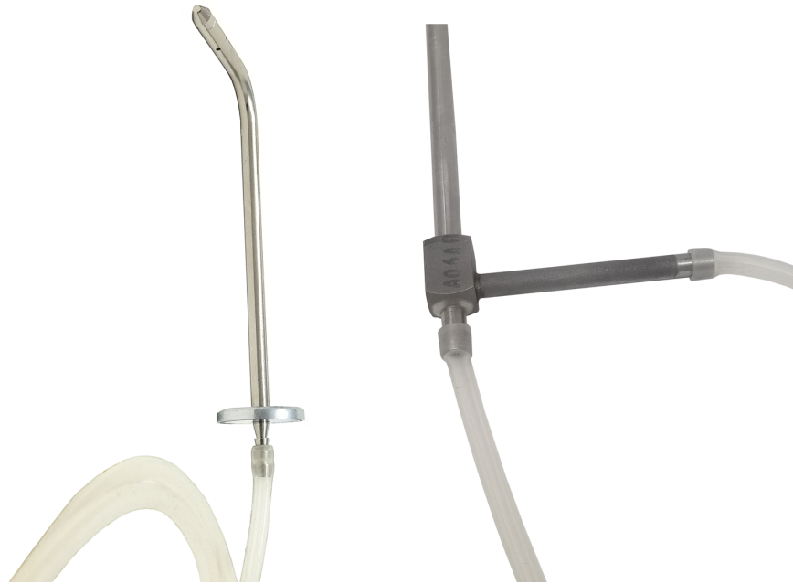
Figure 19 3 mm silicone rubber tubing connected to static pressure tip (left); pitot tube (right). (Rod Lidstone) CC BY ( https://creativecommons.org/licenses/by/4.0/ )
