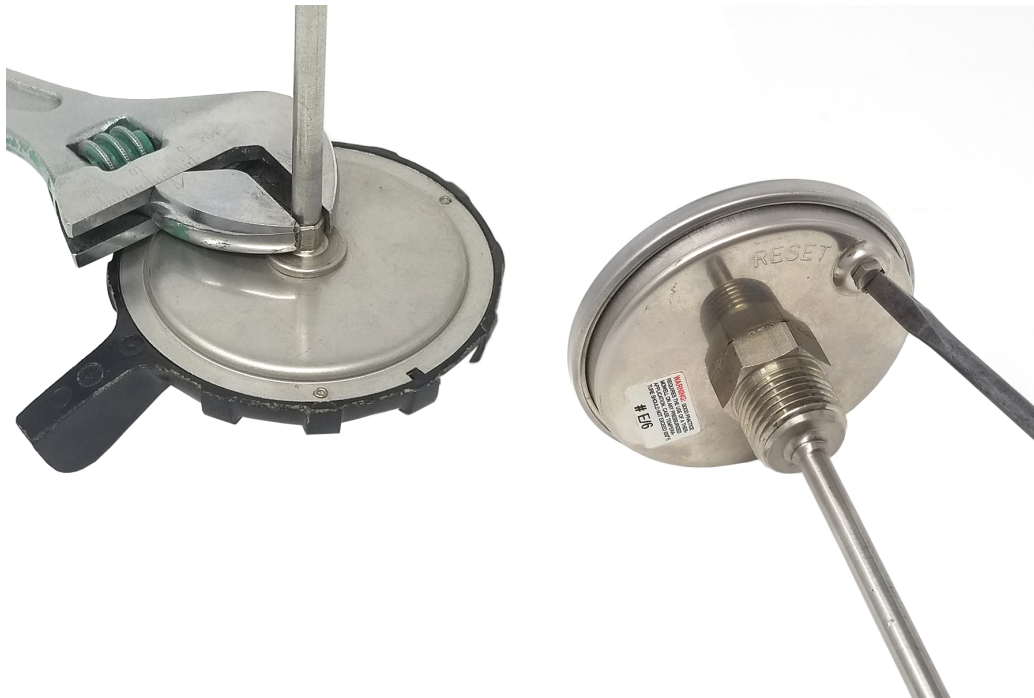
Figure 15 Calibrating analogue dial thermometers. (Rod Lidstone) CC BY ( https://creativecommons.org/licenses/by/4.0/ )
