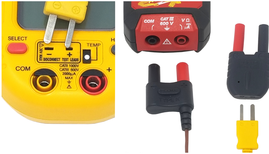
Figure 12 Type k thermocouple connections. (Rod Lidstone) CC BY ( https://creativecommons.org/licenses/by/4.0/ )
