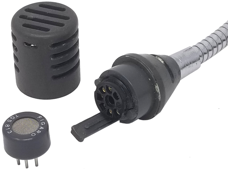
Figure 2 Sensor head disassembled, replaceable sensor lower left. (Skilled Trades BC, 2021) Used with permission.
