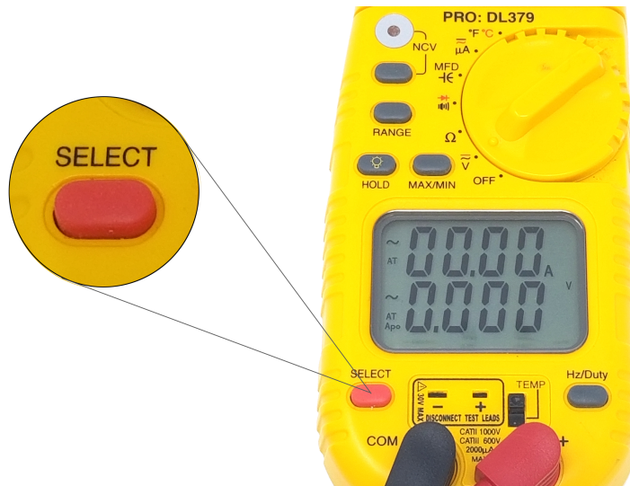
Figure 4 Switching from AC to DC using the SELECT button. (Skilled Trades BC, 2021) Used with permission.
