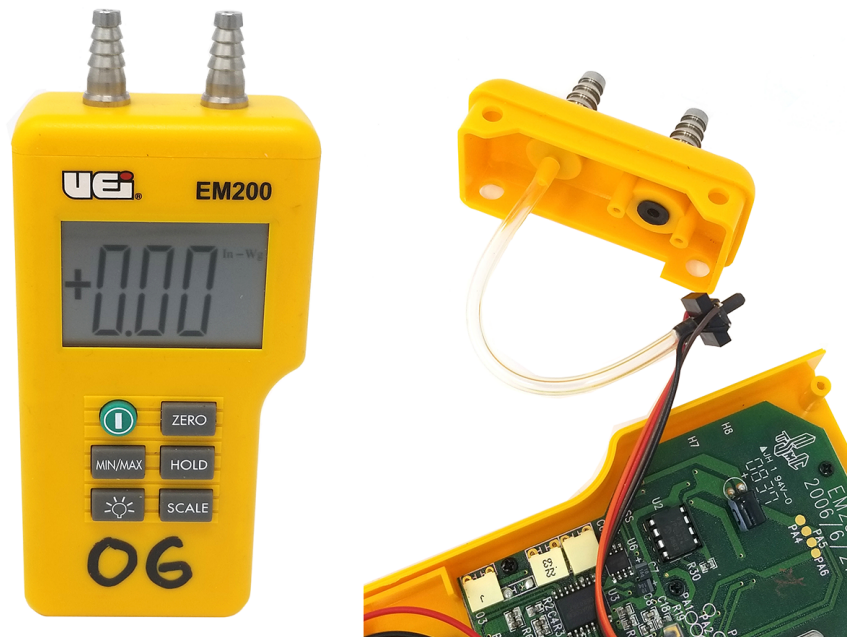
Figure 12 Zeroed electronic manometer (left) disassembled (right). (Rod Lidstone) CC BY ( https://creativecommons.org/licenses/by/4.0/ )
