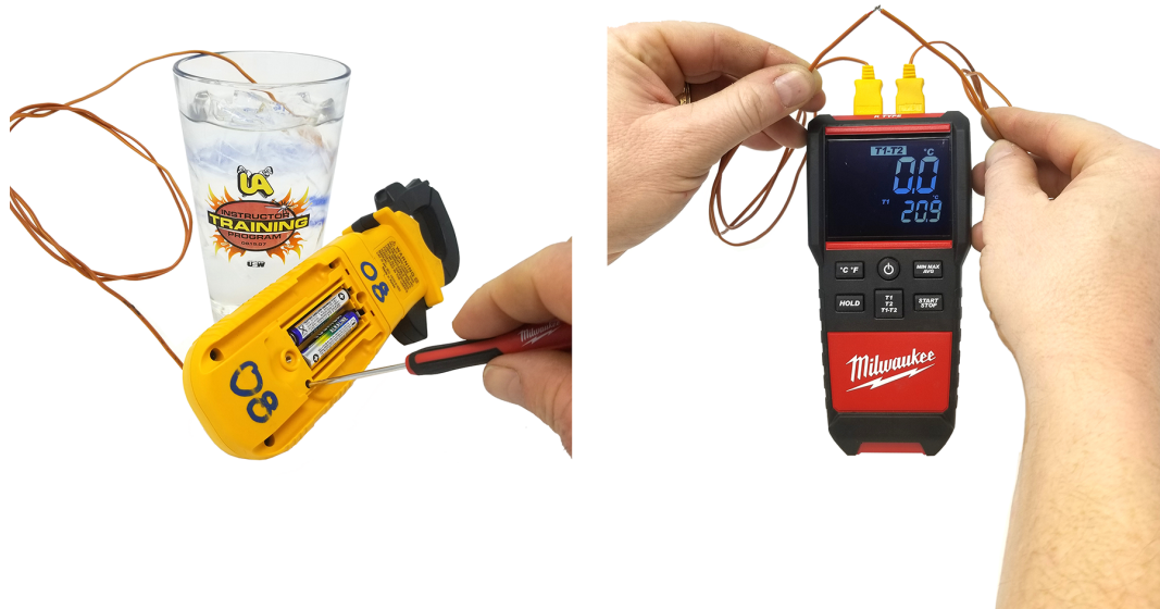
Figure 16 Calibrating DMM temperature readings. (Rod Lidstone) CC BY ( https://creativecommons.org/licenses/by/4.0/ )
