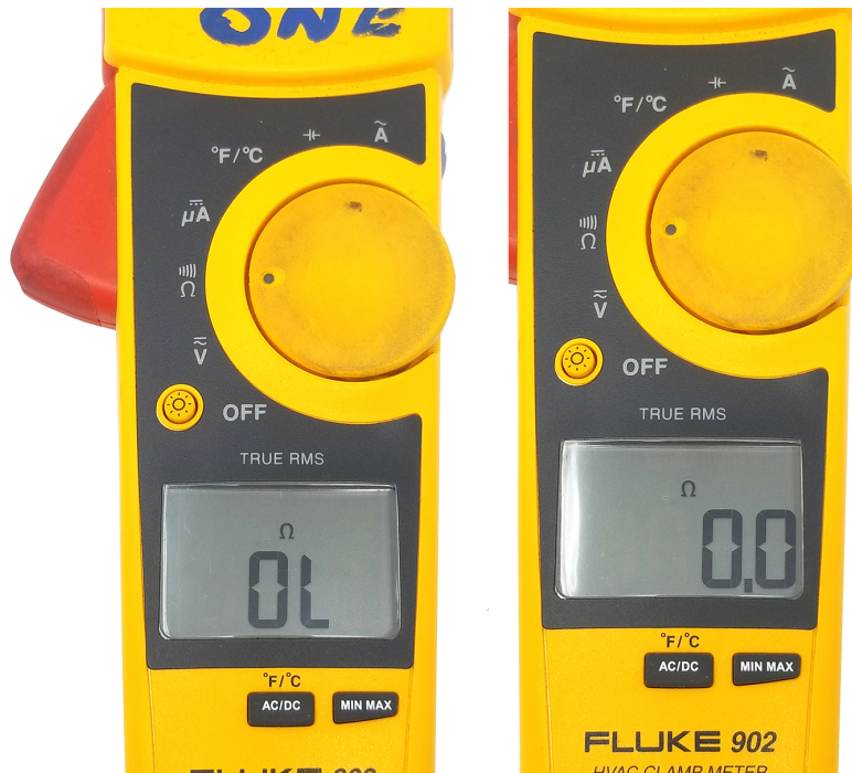
Figure 6 DMM resistance readings; faulty fuse (left), and good fuse (right). (Skilled Trades BC, 2021) Used with permission.
