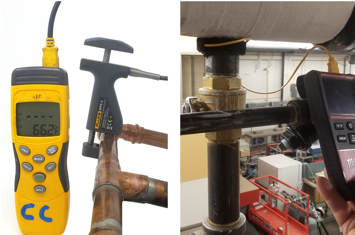
Figure 17 Pipe clamp thermocouples. (Rod Lidstone) CC BY ( https://creativecommons.org/licenses/by/4.0/ )
