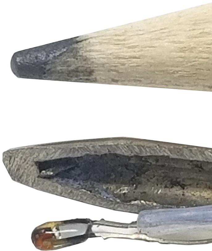
Figure 6 Cutaway of RTD probe. (Rod Lidstone) CC BY ( https://creativecommons.org/licenses/by/4.0/ )
