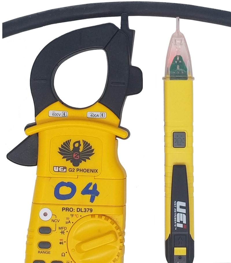
Figure 11 Using non-contact voltage testers. (Skilled Trades BC, 2021) Used with permission.
